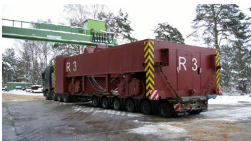
Transportation of a machine part (75 tons)
