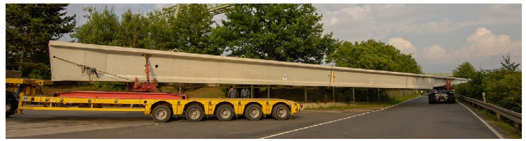
Transportation of overlong concrete parts (up to 50 m and 100 tons)
