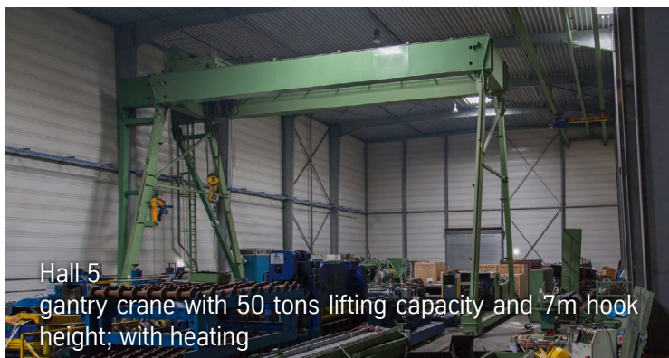
Hall 5: gantry crane with 50 tons lifting capacity and 7m hook height
