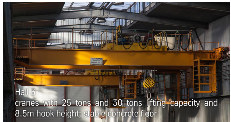
Hall 3 cranes with 25 tons and 30 tons lifting capacity and 8.5m hook height; stable concrete floor
